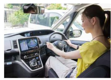
Have you had the experience where you park your car within the correct space but had no room to open the door? The system is reliable in that it shows the guiding lines to indicate the distances necessary to open and close the rear doors.
