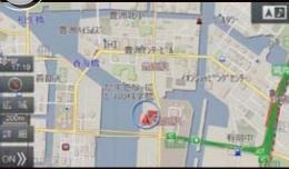
Employs a WXGA LCD, which is 2.4 times as beautiful as the conventional WVGA LCD. In addition to the high resolution, the LCD screen features a "gapless structure", which can clearly display the maps and videos.
