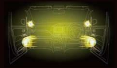
The tweeters are separate units. By adjusting the installation positions, the acoustic space can be improved.
