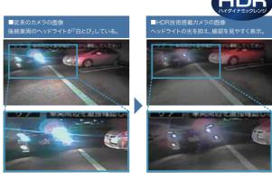
The back camera employs High Dynamic Range (HDR) technology to reduce halation and black defects. Too strong a light from the headlights of the following vehicle is adjusted for an easier view.
