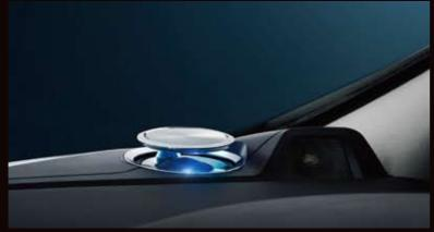
When the ignition is turned on, the active top covers and the tweeters are automatically lifted up. The high sound range from the tweeters reflects to the active top covers, causing the sound to diffuse from the dashboard.
